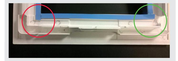
The correct way to apply sealing tape is to always start applying tapes to all horizontal edges, then apply the vertical tapes as shown on picture below, ensuring that the edges of the tape meet, this way when pressure is applied the adhesive will wet into itself and create an excellent long term weather seal. Always refer to our recommended glazing instructions.
